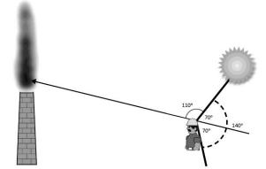
Chapter 5 Figure 2: Determining Proper Sun Position – Vertical Sun Angle
