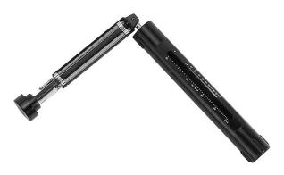
Sling psychrometers are used to determine the temperature and relative humidity.
