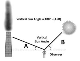
Chapter 8 Figure 2: Abney levels are used to determine vertical viewing angle.
